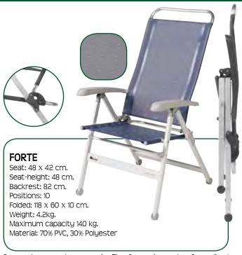
Super strong and ergonomic. The frame is made of anodized aluminum reinforced square tube. The armrests are made of fiberglass reinforced nylon plastic.
