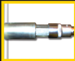
Fig 3. Adjust the height of the corner steady by inserting the 17mm hexagon key into the exposed end of the inner sleeve. Wind up / down with a wheel brace then remove hexagon key.
