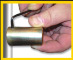
Fig 1. Remove inner sleeve from locking outer cover by inserting a lock key and turning anti-clockwise.
