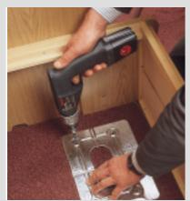
Remove the safe and use the mounting plate as a template to mark where the holes have to be drilled.
