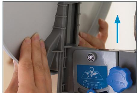
1. To remove 40cm Dish Assembly, press blue catch whilst lifting dish.
