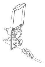
Raise the lid, clean both the water socket and the plug of the pump assembly.
