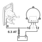
The Ultraflow Filter Housing (9) connects directly to the Truma Smart Switch (11).
