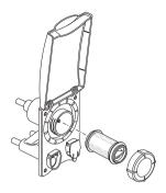
After installation, please drain off the first litres until the filtrate is clear.
