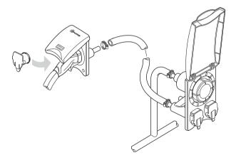
The blanking plug must be fitted to blank off the unused Compact or Filter system.
