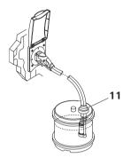
To remove the pump assembly from the Ultraflow Compact Housing, pull the lower trigger and pull out the hose plug.
