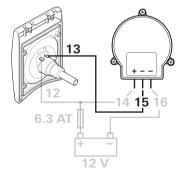
For the winter use, both housings must be connected directly to the Truma Smart Switch.
