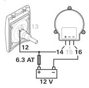
The Ultraflow Compact Housing (13) connects directly to the Truma Smart Switch (15).
