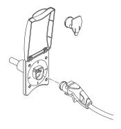
Plug the pump connector into the socket.
