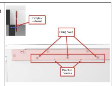
**D** Fit vertical trims with 3 screws using the clearance holes, select holes relevant to the cabinet installation.
