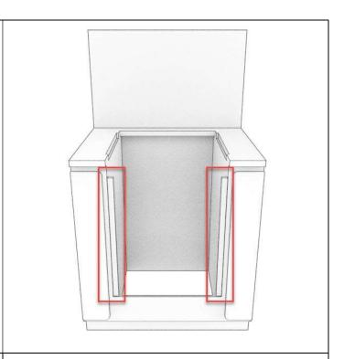
B Fold the supplied installation gauge (as indicated) and mark the trim positions, using the front edge of the worktop as reference on both sides of the cabinet.
