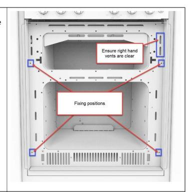
K Lift the appliance lid and use screws appropriate for the installation (12mm+ long screws) to fix the appliance horizontally into the worktop plates.
